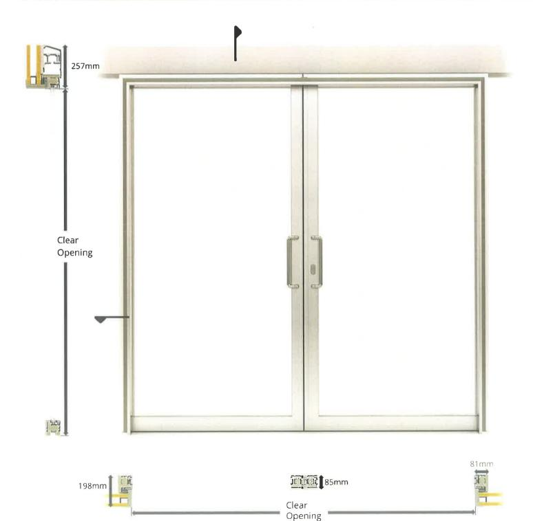
PRODUCT: SOUND REDUCTION: MAX LEAF: 1185\*2162mm FIRE CLASS: MAX GLASS: 1091\*2068mm **DOUBLE LEAF** A60 UP TO 38-40 dB OVERALL C.O.: 2097\*2165mm **SLIDING DOOR**
